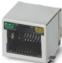
RJ45 PCB connector, number of positions: 8, 10 Gbps, SMD soldering, degree of protection: IP20, connection method: SMD reflow, Tape and Reel
