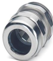
Cable gland, material for screw connection: Brass, nickel-plated, application: EMC, external cable diameter 5 mm ... 10 mm, shielding: yes, connecting thread: M16 x 1.5, color: silver-colored, with O-ring
