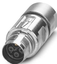
M17, Coupler connector, series: M17 PRO, straight, shielded: yes, for standard and ONECLICK fast locking system, No. of pos.: 3+PE, contact connection type: Socket, Crimp connection, cable diameter range: 3.5 mm ... 6.5 mm, Item is lead-free in accordance with RoHS II without Exemption 6c (Pb < 0.1 %)
