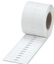
Label, can be removed, can be ordered: by line, white, labeled according to customer specifications, mounting type: adhesive, text field height: 4 mm, text field width: 24 mm
