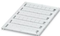
Marker for terminal blocks, Sheet, white, unmarked, can be labeled with: BLUEMARK E.CARD, BLUEMARK ID COLOR, BLUEMARK ID, BLUEMARK CLED, THERMOMARK PRIME 2.0, THERMOMARK PRIME, THERMOMARK CARD 2.0, THERMOMARK CARD, TOPMARK NEO, TOPMARK LASER, mounting type: latching, for terminal block width: 8.2 mm, Number of individual labels: 42, text field height: 10.5 mm, text field width: 7.6 mm
