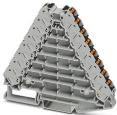
Potential distributors, nom. voltage: 250 V, nominal current: 17.5 A, connection method: Push-in connection, 1st, 2nd, 3rd, 4th, 5th, 6th, 7th and 8th level, Rated cross section: 1.5 mm<sup>2</sup>, cross section: 0.14 mm<sup>2</sup> - 2.5 mm<sup>2</sup>, mounting: NS 35/7,5, NS 35/15, color: gray, color of connection elements: black
