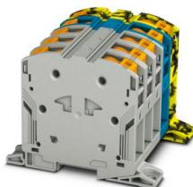
High-current terminal block, Blocked, nom. voltage: 1000 V, nominal current: 232 A, number of connections: 10, number of positions: 5, connection method: PowerTurn connection, cross section: 25 mm<sup>2</sup> - 95 mm<sup>2</sup>, mounting type: direct screw connection, color: gray/blue/black-yellow
