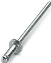
Blind rivets, Ø 2.4 mm, 8 mm sleeve length, aluminum sleeve, zinc-plated steel pin, special version with extended pin for fixing UW/RW/PW 4... (the UNIFOX-RVT M/BIT 2,4L nosepiece is required for processing)
