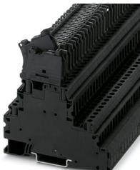
Fuse modular terminal block, fuse type: Glass / ceramics / ..., fuse type: G / 5 x 20, nom. voltage: 60 V, Thermal continuous current  $I_{th}$ : 28 A, connection method: Screw connection, Rated cross section: 4 mm<sup>2</sup>, cross section: 0.14 mm<sup>2</sup>- 6 mm<sup>2</sup>, connection method: Screw connection, Rated cross section: 4 mm<sup>2</sup>, cross section: 0.14 mm<sup>2</sup>- 6 mm<sup>2</sup>, mounting type: NS 35/7,5, NS 35/15, color: black
