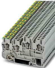
Installation protective conductor terminal block, nom. voltage: 250 V, nominal current: 18 A, number of connections: 4, connection method: Spring-cage connection, Rated cross section: 2.5 mm<sup>2</sup>, cross section: 0.08 mm<sup>2</sup> - 4 mm<sup>2</sup>, mounting type: NS 35/7,5, NS 35/15, color: gray
