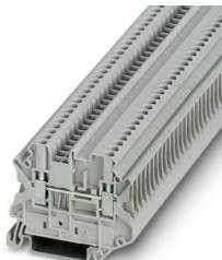
Feed-through terminal block, nom. voltage: 800 V, nominal current: 24 A, number of connections: 2, number of positions: 1, connection method: Screw connection, Rated cross section: 2.5 mm<sup>2</sup>, cross section: 0.14 mm<sup>2</sup> - 4 mm<sup>2</sup>, mounting type: NS 35/7,5, NS 35/15, color: gray
