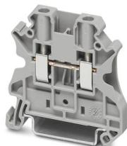
Feed-through terminal block, With breakout partition plate in the bridge shaft, nom. voltage: 1000 V, nominal current: 32 A, number of connections: 2, number of positions: 1, connection method: Screw connection, Rated cross section: 4 mm<sup>2</sup>, cross section: 0.14 mm<sup>2</sup> - 6 mm<sup>2</sup>, mounting type: NS 35/7,5, NS 35/15, color: gray
