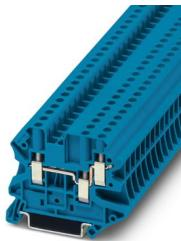
Feed-through terminal block, nom. voltage: 500 V, nominal current: 32 A, number of connections: 3, connection method: Screw connection, Rated cross section: 4 mm<sup>2</sup>, cross section: 0.14 mm<sup>2</sup> - 6 mm<sup>2</sup>, mounting type: NS 35/7,5, NS 35/15, color: blue
