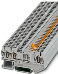
Knife-disconnect terminal block, nom. voltage: 400 V, nominal current: 20 A, connection method: Spring-cage connection, Rated cross section: 2.5 mm<sup>2</sup>, cross section: 0.08 mm<sup>2</sup> - 4 mm<sup>2</sup>, mounting: NS 35/7,5, NS 35/15, color: gray
