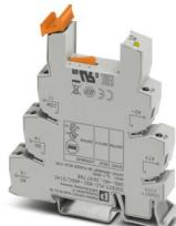
14 mm PLC basic terminal block for high continuous currents with screw connection, without relay or solid-state relay, for mounting on DIN rail NS 35/7,5, 1 changeover contact, input voltage 48 V DC
