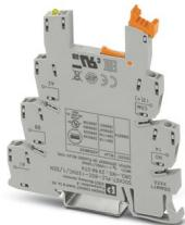
6.2 mm PLC basic terminal block for input functions with screw connection, without relay or solid-state relay, for mounting on DIN rail NS 35/7,5, with sensor supply voltage distribution (BB), 1 N/O contact, input voltage 120 V AC/DC
