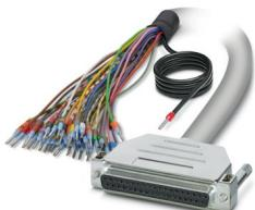
Assembled shielded round cable; connection 1: Single wires (37-position) (The wires are marked and fitted with ferrules. The braided shield is routed to a separate cable end.); connection 2: D-SUB socket strip (1x 37-position); cable length: 20 m
