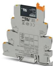
PLC-INTERFACE for input functions, consisting of PLC-BPT.../SEN basic terminal block with push-in connection and plug-in miniature solid-state relay, for mounting on DIN rail NS 35/7,5, 1 N/O contact, input: 120 V AC/110 V DC, output: 3 - 48 V DC/100 mA
