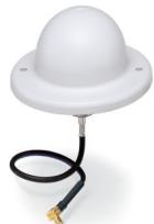
Omnidirectional antenna with protection against vandalism, 2.4 GHz, gain: 3 dBi, polarization: linear, opening angle: h/v 360°/85°, degree of protection: IP55, connection: MCX (male), for control cabinet mounting (optional panel mounting), incl. 1.5 m / 5 ft. connecting cable
