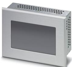
Touch panel, 10.92 cm / 4.3"-TFT display (analog resistive (polyester)), 480 x 272 pixel(s) (WQVGA), 65536 colors, Arm9™, 200 MHz, 2x USB Host 2.0, 1x COM (RS-232/485), 1 x Ethernet (10/100 Mbps), RJ45, Windows® CE 5.0, TSvisRT, without bus system.
