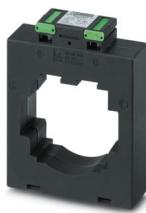
Window-type current transformer, 1,500 A AC primary current; 5 A AC secondary current; accuracy class 1; 15 VA rated power
