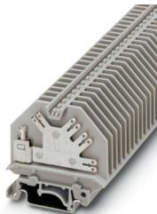
Feed-through terminal block, nom. voltage: 800 V, nominal current: 32 A, 1st level connection left, connection method: Screw connection, Rated cross section: 4 mm<sup>2</sup>, cross section: 0.2 mm<sup>2</sup> - 4 mm<sup>2</sup>, connection method: Spade connection, mounting: NS 35/7,5, NS 35/15, NS 32, color: gray
