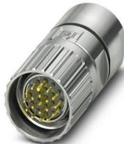
M23, Cable connector, series: M23 PRO, straight, shielded: yes, Screw locking mechanism, No. of pos.: 16+2+PE, Direction of rotation: Standard, contact connection type: Pin, Crimp connection, cable diameter range: 3 mm ... 15 mm, coding: N, Item is lead-free in accordance with RoHS II without Exemption 6c (Pb < 0.1 %)
