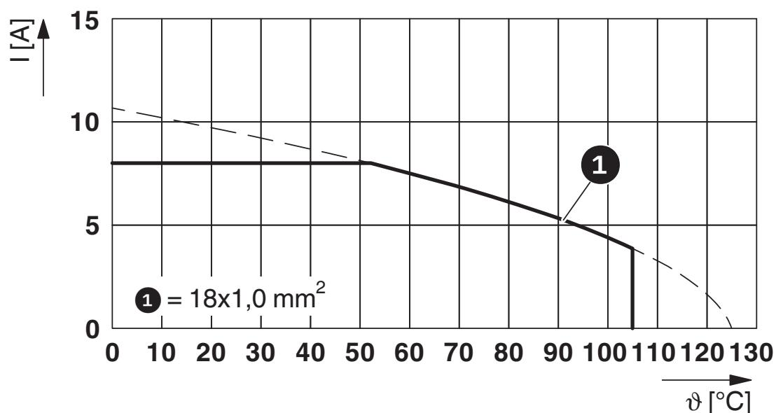
$I$  = current strength,  $\vartheta$  = ambient temperature,  $18 \times 8$  A
