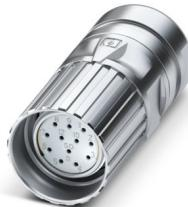
M23, Cable connector, series: CA, straight, shielded: yes, Screw locking mechanism, No. of pos.: 12, Direction of rotation: Counter direction, contact connection type: Socket, Crimp connection, cable diameter range: 6 mm ... 10 mm, coding: N, this item is expected to be lead-free from Q2 2026 in accordance with RoHS II without exception 6c (Pb < 0.1%), a lead-free alternative is possible on request in advance
