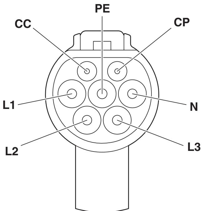
Pin assignment of the Vehicle Connector
