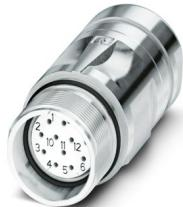
M23, Coupler connector, series: CA, straight, shielded: yes, for standard and SPEEDCON interlock, No. of pos.: 16, Direction of rotation: Standard, contact connection type: Socket, Crimp connection, cable diameter range: 3 mm ... 14.5 mm, coding: N, this item is expected to be lead-free from Q1 2026 in accordance with RoHS II without exception 6c (Pb < 0.1%), a lead-free alternative is possible on request in advance
