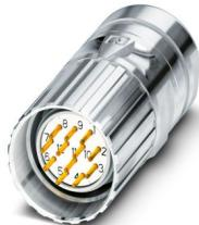
M23, Cable connector, series: CA, straight, shielded: yes, Screw locking mechanism, No. of pos.: 16, Direction of rotation: Standard, contact connection type: Pin, Crimp connection, cable diameter range: 6 mm ... 10 mm, coding: N, this item is expected to be lead-free from Q2 2026 in accordance with RoHS II without exception 6c (Pb < 0.1%), a lead-free alternative is possible on request in advance
