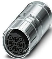
Cable connector, straight long, Screw locking mechanism, M40, number of positions: 2+3+PE, contact connection type: Socket, shielded: yes, degree of protection: IP67, cable diameter range: 9 mm ... 14 mm, number of positions: 6, connection method: Crimp connection, series: SM, this item is expected to be lead-free from Q3 2026 in accordance with RoHS II without exception 6c (Pb < 0.1%), a lead-free alternative is possible on request in advance
