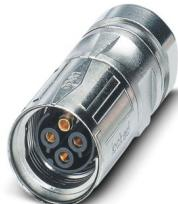
Cable connector, straight, SPEEDCON, M17, number of positions: 5+PE, contact connection type: Socket, shielded: yes, degree of protection: IP67, cable diameter range: 5 mm ... 8 mm, number of positions: 6, connection method: Crimp connection, series: ST, this item is expected to be lead-free from Q3 2025 in accordance with RoHS II without exception 6c (Pb < 0.1%), a lead-free alternative is possible on request in advance
