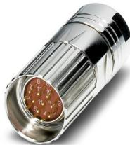
Cable connector, straight, Screw locking mechanism, M23, number of positions: 17, contact connection type: Pin, shielded: yes, cable diameter range: 6 mm ... 10 mm, number of positions: 17, connection method: Crimp connection, series: RF
