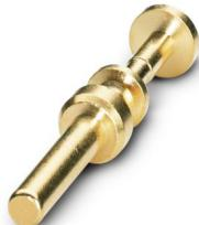
Crimp contact, Pin, turned, contact diameter: 3.6 mm, connection cross section: 4 mm<sup>2</sup> ... 6 mm<sup>2</sup>, contact material: CuZn, Alternative product in accordance with RoHS II without Exemption 6c (Pb < 0.1 %) item no.: 1241971
