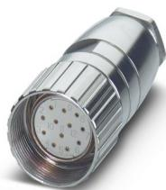
M23, Cable connector, series: RC, straight, shielded: no, Screw locking mechanism, No. of pos.: 12, Direction of rotation: Standard, contact connection type: Socket, Solder cup, coding: N
