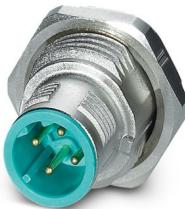
Device connector rear mounting, Ethernet CAT5 (100 Mbps), 4-position, Pin, straight, M12-SPEEDCON, D-coding, Wave soldering, this item is expected to be lead-free from Q1 2026 in accordance with RoHS II without exception 6c (Pb < 0.1%), a lead-free alternative is possible on request in advance
