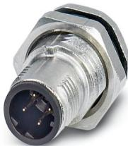
Device connector rear mounting, 4-position, Pin, straight, M12-SPEEDCON, D-coding, Wave soldering, this item is expected to be lead-free from Q1 2026 in accordance with RoHS II without exception 6c (Pb < 0.1%), a lead-free alternative is possible on request in advance
