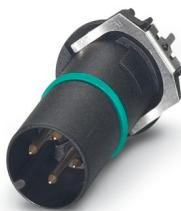
Contact carrier, Universal, 4-position, Pin, straight, M12, A-coding, THR solder connection, Item is lead-free in accordance with RoHS II without Exemption 6c (Pb < 0.1 %)
