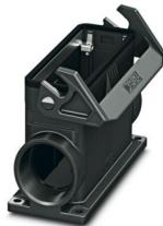
Surface mounting housing B24, with single locking latch, material: PA 6.6-FR, cable outlets: 2, lateral, 2x M32, height: 84 mm, cable gland: none, Standard, including 2x reducing adapter
