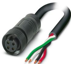
Power cable, 4-position, PVC, black, free cable end, on Socket straight 7/8"-16UNF, coding: A, cable length: 1 m
