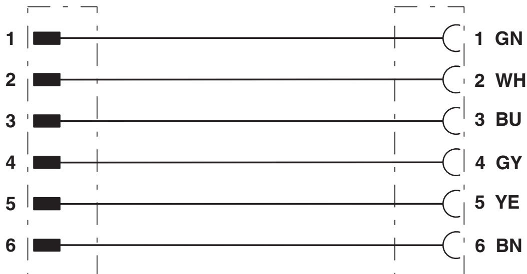
Contact assignment of 7/8" plugs/sockets
