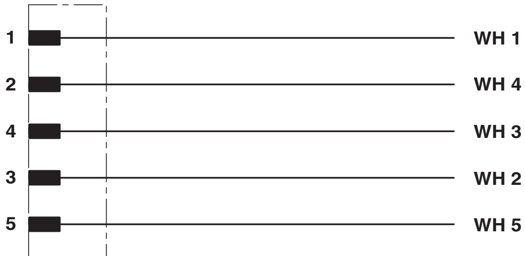
Contact assignment of the M12 plug
