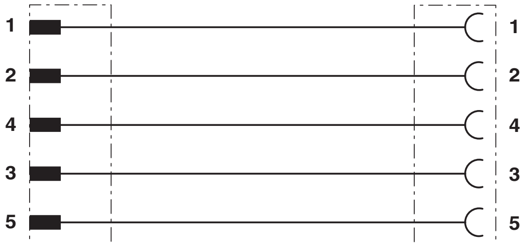
Contact assignment of M8 plugs/sockets
