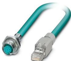
Assembled Ethernet cable, shielded, 4-pair, AWG 26 suitable for use with drag chain (19-wire), RAL 5021 (sea blue), M12 flush-type socket, rear wall/screw mounting with M16 thread on RJ45 connector/IP20, line, length 1 m
