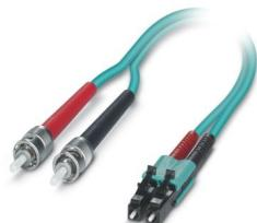
Assembled FO cable, zip cord cable, multi-mode fiberglass 50/125  $\mu\text{m}$ , OM3, plug: LC/B-FOC (ST), degree of protection: IP20, for installation in cable ducts or control cabinets, length: 2 m
