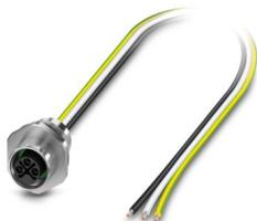
Device connector front mounting, Power, 3-position, Flush-type female connector, straight, M12-Standard, S-coding, on free cable end, Individual wires, cable length: 2 m, 2.50 mm<sup>2</sup>, PEX litz wire
