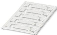
Marker for end clamp, Sheet, white, unmarked, can be labeled with: BLUEMARK E.CARD, BLUEMARK ID COLOR, BLUEMARK ID, BLUEMARK CLED, THERMOMARK PRIME 2.0, THERMOMARK PRIME, THERMOMARK CARD 2.0, THERMOMARK CARD, TOPMARK NEO, TOPMARK LASER, mounting type: latching, for terminal block width: 9.4 mm, Number of individual labels: 5, text field height: 8 mm, text field width: 30 mm
