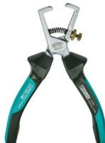
Stripping pliers, for removing the sheath from cables up to 5 mm in diameter, for stripping conductors with a cross section of up to 10 mm<sup>2</sup>, scale for measuring the stripping length; VDE-tested.
