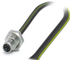
Device connector rear mounting, Power, 6-position, Pin, straight, M12-Standard, M-coding, on free cable end, Individual wires, cable length: 1.5 m,  $1.31 \text{ mm}^2$ , UL/cUL stranded hook-up wire, potted, this item is expected to be lead-free from Q1 2026 in accordance with RoHS II without exception 6c (Pb < 0.1%), a lead-free alternative is possible on request in advance
