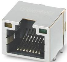
RJ45 PCB connector, number of positions: 8, 10 Gbps, Wave soldering, degree of protection: IP20, connection method: THT wave, Tray
