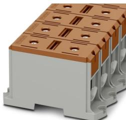
High-current terminal block, nom. voltage: 1000 V, nominal current: 380 A, number of connections: 2, number of positions: 1, connection method: Screw connection, Rated cross section: 240 mm<sup>2</sup>, cross section: 35 mm<sup>2</sup> - 240 mm<sup>2</sup>, Rated cross section: 240 mm<sup>2</sup>, cross section: 35 mm<sup>2</sup> - 240 mm<sup>2</sup>, mounting type: Screw mounting, color: brown
