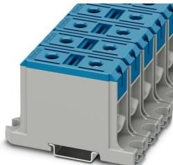
High-current terminal block, nom. voltage: 1000 V, nominal current: 220 A, number of connections: 2, number of positions: 1, connection method: Screw connection, Rated cross section: 95 mm<sup>2</sup>, cross section: 16 mm<sup>2</sup> - 95 mm<sup>2</sup>, Rated cross section: 95 mm<sup>2</sup>, cross section: 16 mm<sup>2</sup> - 95 mm<sup>2</sup>, mounting type: NS 35/15, NS 35/7,5, color: blue
