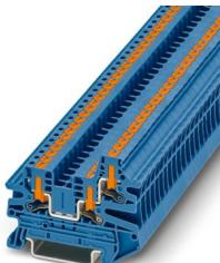
Feed-through terminal block, nom. voltage: 800 V, nominal current: 24 A, number of connections: 3, connection method: Push-in connection, Rated cross section: 2.5 mm<sup>2</sup>, cross section: 0.14 mm<sup>2</sup> - 4 mm<sup>2</sup>, mounting type: NS 35/7,5, NS 35/15, color: blue
